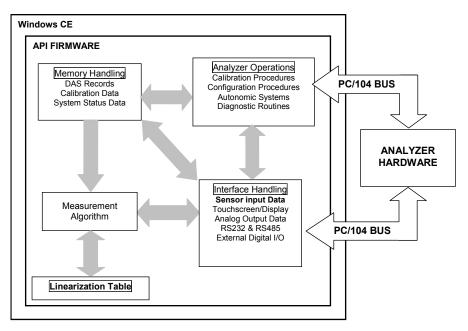
Figure 13-18: Basic Software Operation
